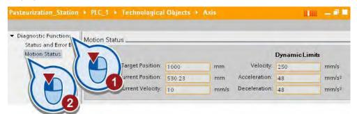
The current position of the motor axis is shown in the "Current position" field. When the target position of 500 mm relative to the start position is reached, the axis is set to stop.
