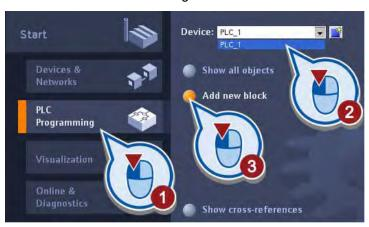
3. Create a cyclic interrupt OB with the name "PID". Make sure that the "Add new and open" check box is selected.
