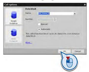
The data block ""IEC\_Timer\_0" is created in the "Programming blocks" folder and assigned to the instruction "On delay". The data of the inserted time instruction are stored in this data block.
