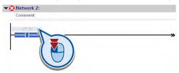
4. Interconnect the normally open contact with the tag "ON".
