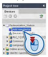
2. Assign a name and select an HMI device. Leave the "Start device wizard" check box selected.
