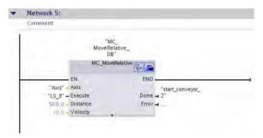
The motion is started when the light barrier "LS3" is activated. When the target position has been reached, the bit of the "start\_conveyor\_2" tag is set at "Done" output, by means of which the second conveyor can be set into motion.
