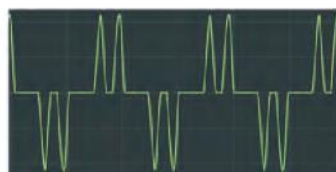
Motor drive without DC choke THDi 107%
