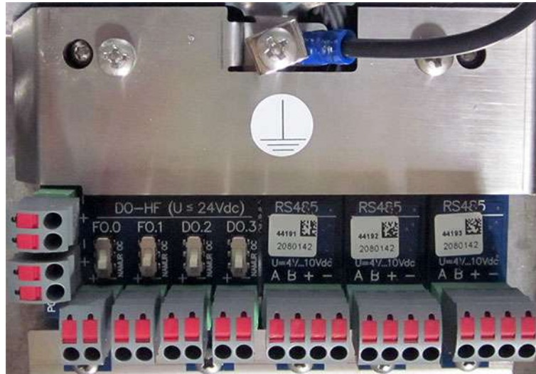
Fig. 42 Terminal assignment Ex-i terminal compartment (example)
