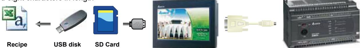
The recipe data can be saved in CSV format and easily edited on an external PC in Excel to effectively save PLC memory.
