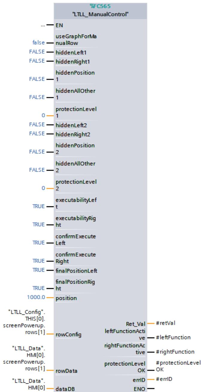
Fig. 7-13: Call interface for block L TLL\_ManualControl
