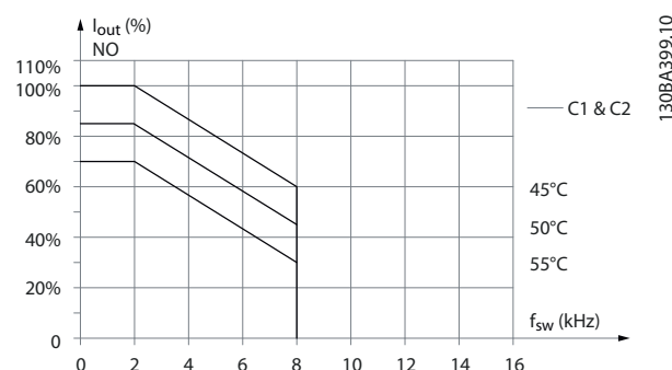
Figure 5.17 Derating of I out for Different T AMB, MAX for Enclosure Sizes C1 and C2, using SFAVM in Normal Overload Mode (110% Over Torque)
