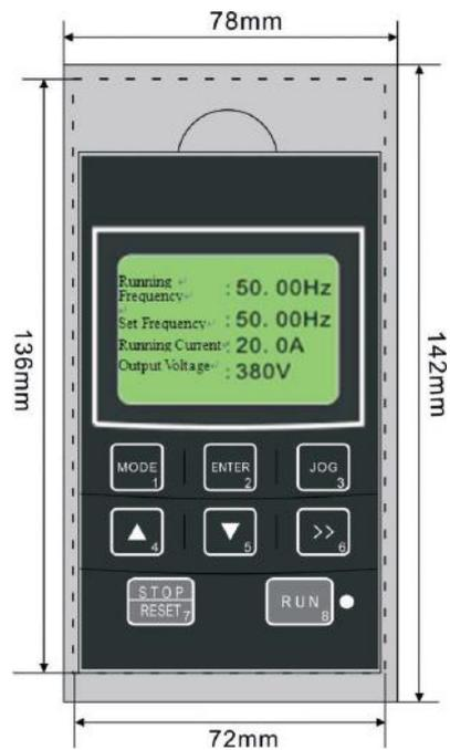
Installation dimension of Keyboard Booth: 136\*72mm      Outer dimension of Keyboard Booth: 142\*78mm
