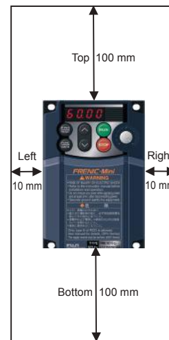
Figure 2.1 Mounting Direction and Required Clearances
