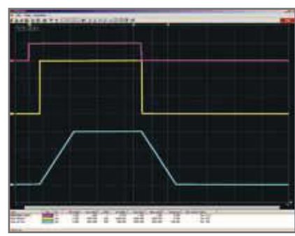
Speed cycle Start, ramp reference 1500 rpm, ramp output reaches 1500 rpm, Stop, ramp reference 0 rpm, ramp output reaches 0 rpm.
