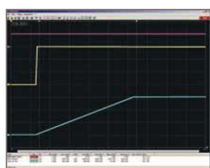
Zoom Ramp output phase from 0 rpm to 1500 rpm of the previous cycle.
