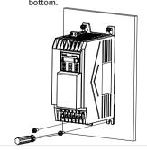
Step 3 Preload the two screws at the Step 4 Tighten the four preloaded screws.
