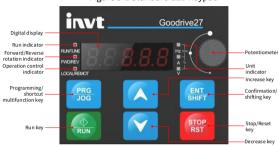
Figure 5-1 Standard LED keypad
