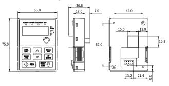
Figure D-5 Keypad openings without a bracket
