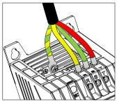
Step 2 Connect the yellow and green grounding line of the motor cable to the VFD PE terminal, connect the motor 3PH cable to the U, V, and W terminals, and tighten up.
