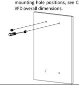
Step 1 Mark the mounting hole positions, Step 2 Fasten the VFD end with the hardy holes onto the two preloaded screws.
