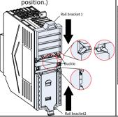
vertically on the DIN rail, and push sheet metal lock catch upwards to make it tightly engage with the rail.
