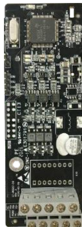
24V simplified incremental PG card EC-PG507-24
