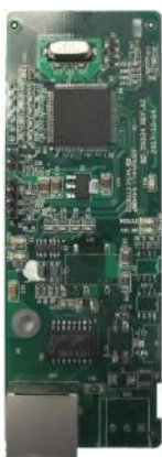
Ethernet communication card EC-TX504
