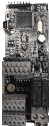
Programmable expansion card EC-PC502-00
