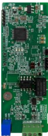
CAN multi-protocol communication card EC-TX505C
