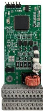
24V incremental PG card EC-PG505-24B
