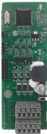
Simplified incremental PG card EC-PG507-12
