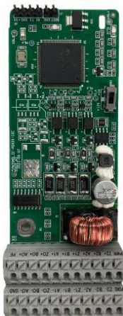
Multifunction incremental PG card EC-PG505-12
