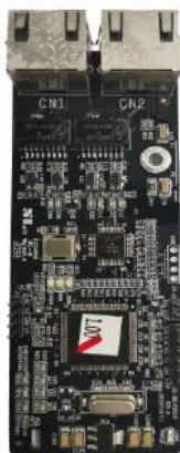
Ethernet/IP communication card EC-TX510/ Modbus TCP communication card EC-TX515
