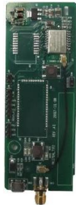
Bluetooth/WIFI communication card EC-TX501/502
