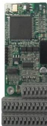
UVW incremental PG card EC-PG503-05
