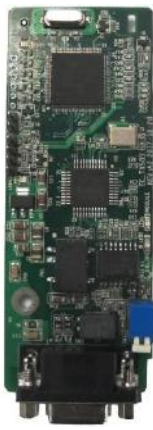
PROFIBUS-DP communication card EC-TX503
