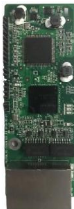
PROFINET communication card EC-TX509
