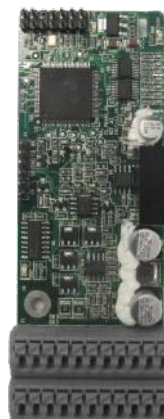
Resolver PG card EC-PG504-00
