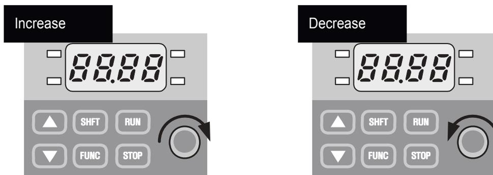
● Frequency setting with the loader's volume resistance(V0)
