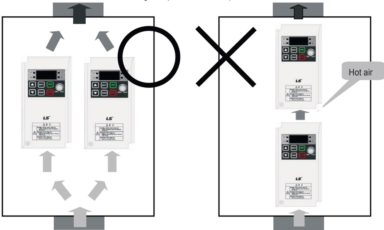
**Caution** Arrange hot air from the inverters is discharged when installing them on a panel. 'X' shows incorrect layout example.
