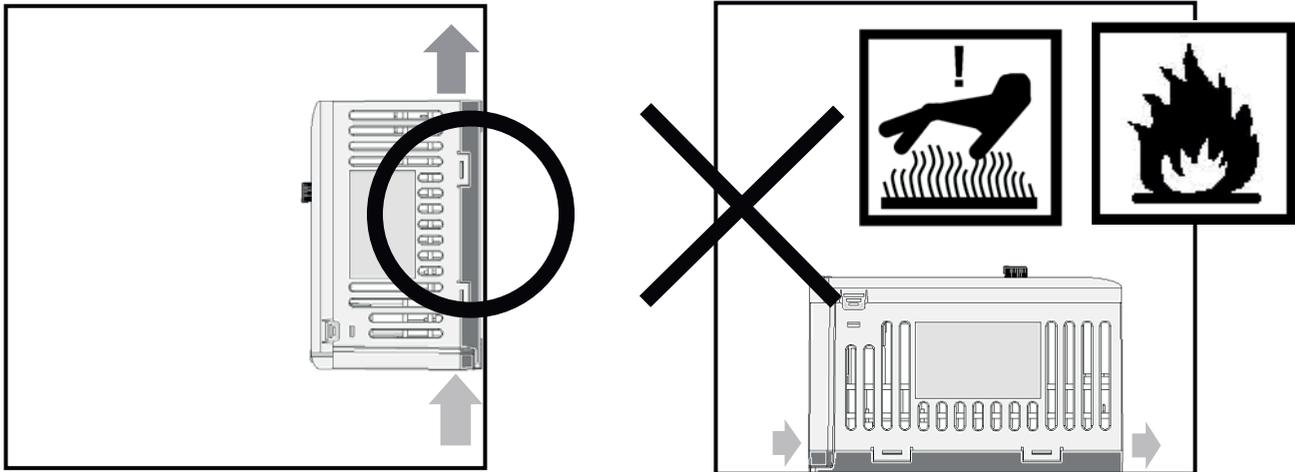
**⚠ Caution** iE5 has self cooling structure using air. Therefore install the inverter vertically possible to air circulation. Malfunction or fire may be caused when installed horizontally.
