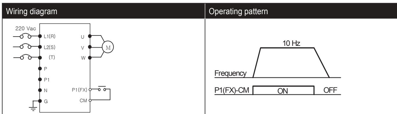
● If setting frequency with volume resistance on the loader and commanding operation on the inverter's terminal
