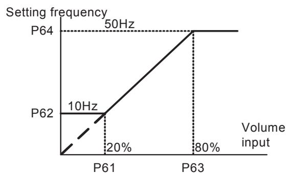
● Frequency setting using AI(analogue input) terminal
