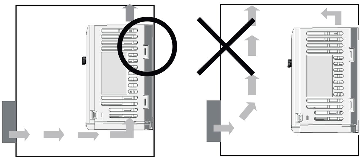
**Caution** A fan is to be installed so that the air inside the inverter is well discharged as seen in the left figure. 'X' shows an example of reduced cooling effect, possibly causing the inverter to overheat.
