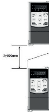
Up and down the installation drawing
