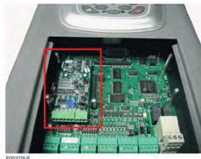
Figure 115: Encoder board fastened to its slot
