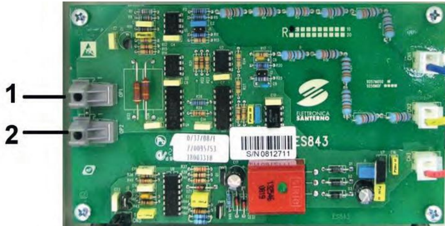
Figure 37: ES843 Bus-bar Voltage Acquisition Board
