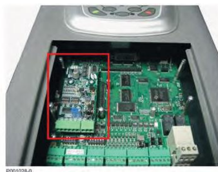
Figure 124: Encoder board fastened to its slot
