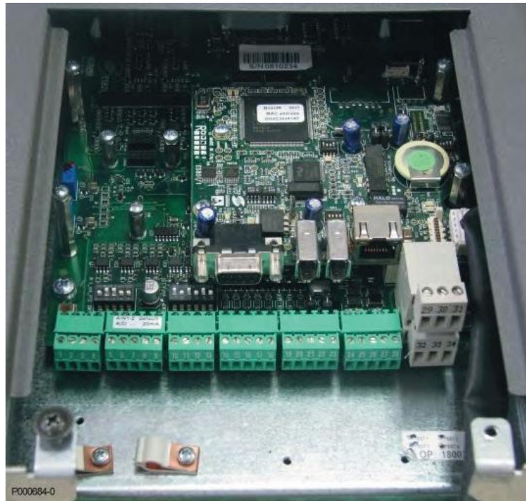
Figure 159: ES851 DataLogger fitted into slot B
