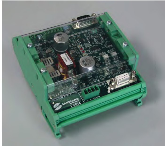
Figure 179: ES914 Power supply unit board
