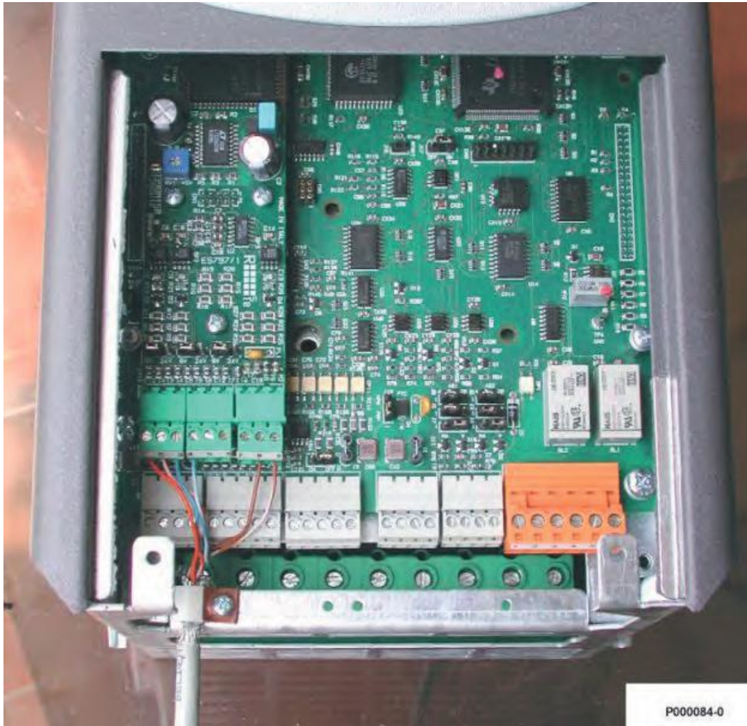
Figure 121: Wiring the encoder cable
