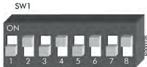
Figure 189: DIP-switch SW1 setting for five-channel mode
