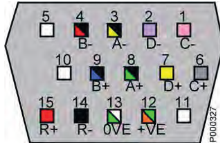
Figure 187: Pin layout on the high density connector
