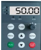
Fig 3-2 Stop Status Parameter Display Display Set Frequency "50.00"
