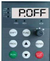
Fig 3-1 Power-on Parameter Display Initialization Display "P.OFF"
