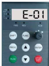
Fig 3-4 Fault Alarm Display of Over current during Accelerating
