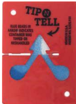
Figure 3-3 Tilt indicator tripped
