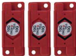
Figure 3-4 Shock indicator tripped
