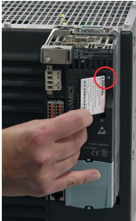
Figure 7-12 CU310-2 DP Inserting the memory card
