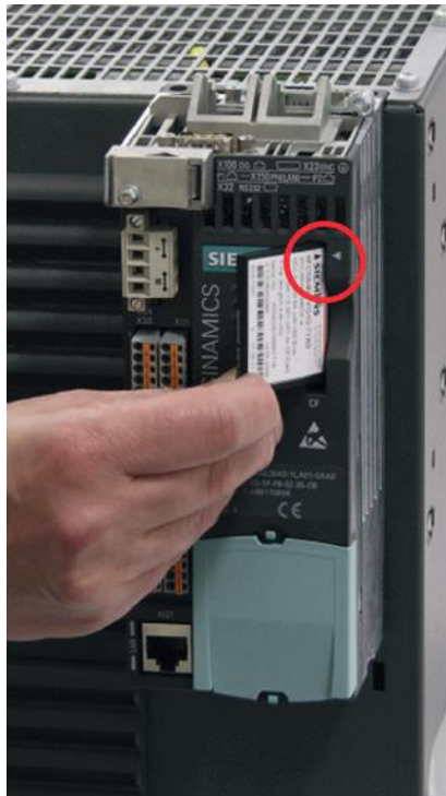
Figure 7-5 CU310-2 PN Inserting the memory card
