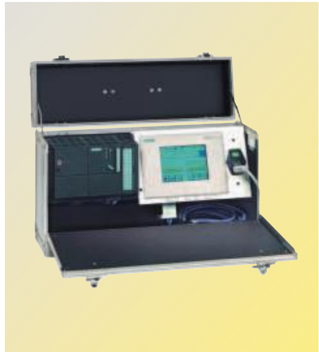
Fig. 5/3 Demonstration case with Drive ES and touch panel
