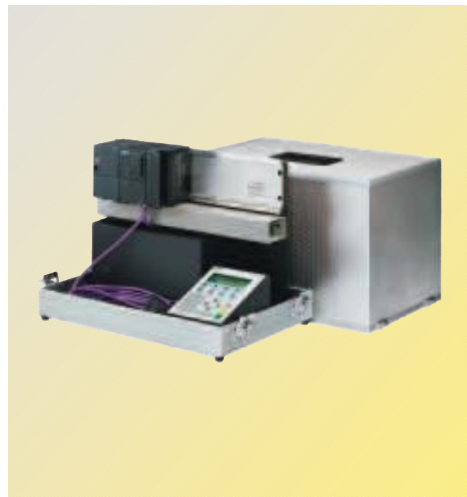
Fig. 5/4 PROFIBUS DP/SIMATIC S7 demonstration case
