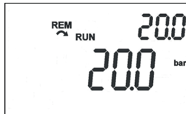
Figure 15.3: Example of HMI in the monitoring mode to use the PID controller
