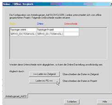
Figure 10-26 ONLINE/OFFLINE comparison, loading into PG
