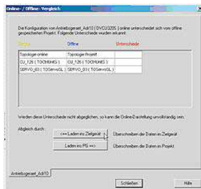
Figure 10-25 ONLINE/OFFLINE comparison, loading into target system
