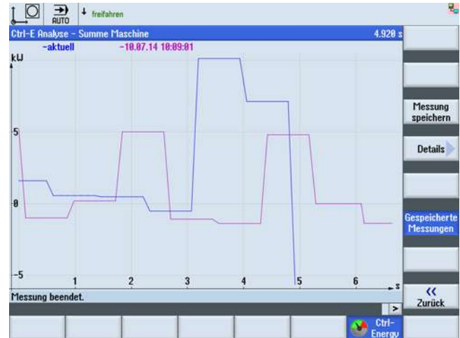
Graphical comparison of two measurements for qualitative evaluation of the energy consumed by a machine tool.
