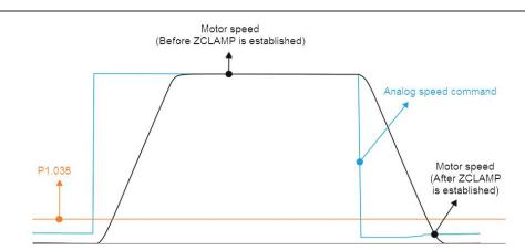
Bit 10 = 1 and command source is the internal register. ZCLAMP function uses the register Speed command with acceleration or deceleration to determine if this function should be enabled. When ZCLAMP conditions are met, the motor speed is set to 0 rpm.
