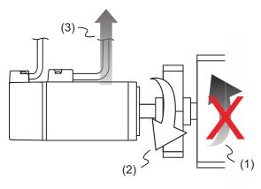
(1) Moving direction of the object; (2) Direction of torque;
