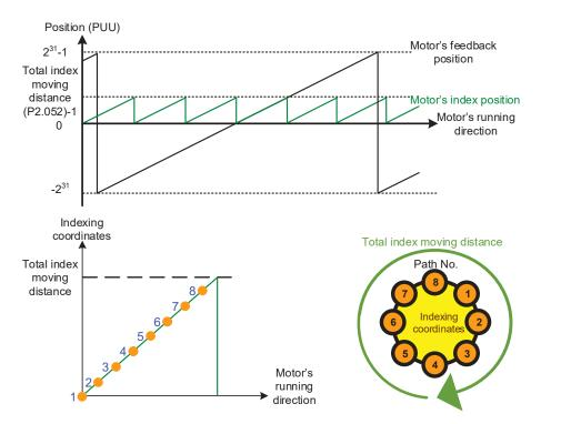
Figure 7.1.3.6.1 PR mode indexing coordinates
