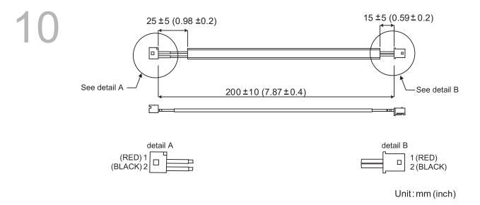
Battery box cable for self-wiring (part number: 3864850600)
