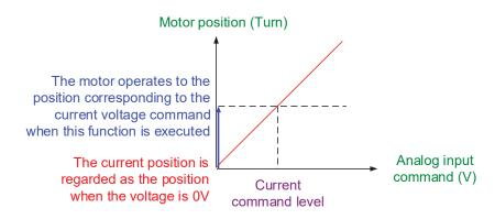
1: after the servo is on, if the command level is not changed, the motor does not operate.
