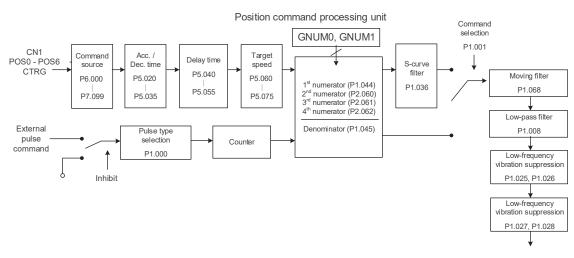
The upper path of the above diagram is the PR mode and the lower one is the PT mode that you can select with P1.001. You can set the E-Gear ratio in both modes to adjust the positioning resolution. In addition, you can use either a moving filter or low-pass filter to smooth the command (described as follows).
