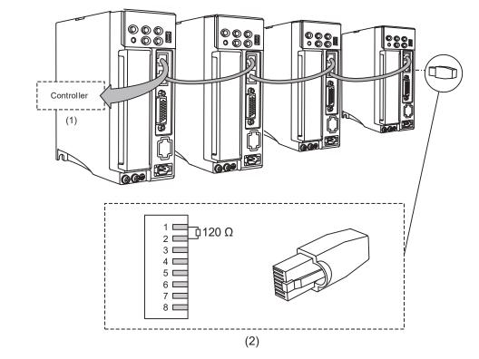
(1) Connect to the controller / PLC; (2) Wiring for CAN terminal resistor
