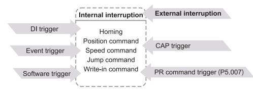
Figure 7.1.6.5 Internal and external interruption
