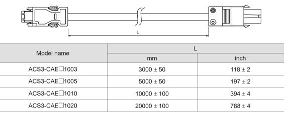
Note: select cables according to the  $\square$  in the model name. F represents flexible cables and N represents
