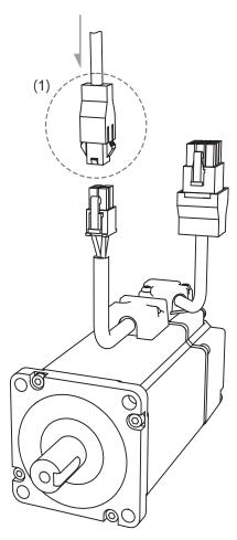
Note: pin assignments of the B3 and B2 models are the same. For easier wiring, the B3's connector illustration (angle of viewing) is changed, which is different from that of B2.
