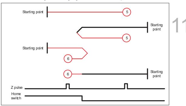
Methods 5 and 6: homing on the falling edge of home switch and Z pulse
