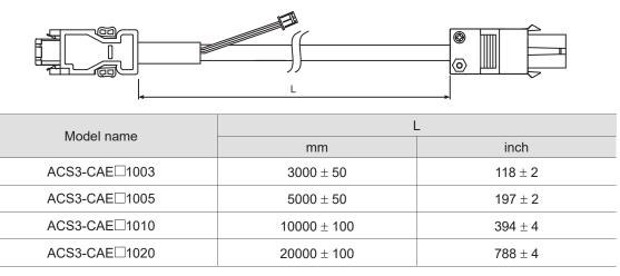
Note: select cables according to the  $\Box$  in the model name. B represents flexible cables and A represents standard cables.
