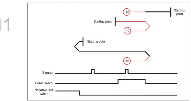
Method 12: homing on the negative limit switch, falling edge of home switch, and Z pulse
