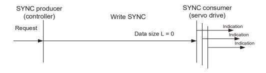
The SYNC object is used to achieve PDO transmission and reception synchronization between the controller and servo drive. The SYNC object transmission cycle is set by the object OD 1006h (see Section 11.4 for detailed settings).
