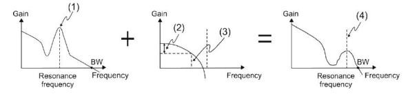
(1) Resonance point; (2) Attenuation rate (-3 dB); (3) Low-pass filter (Cutoff frequency of low-pass filter = 1000 / P2.025 Hz); (4) Resonance point suppressed by the low-pass filter
