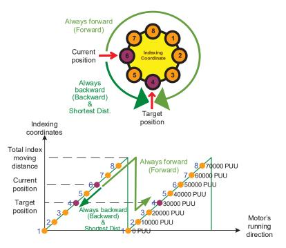
Figure 7.1.3.6.4 Motor's operation direction and indexing coordinates
