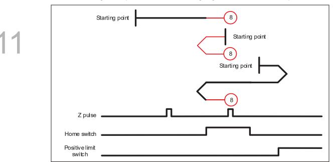
Method 8: homing on the positive limit switch, rising edge of home switch, and Z pulse
