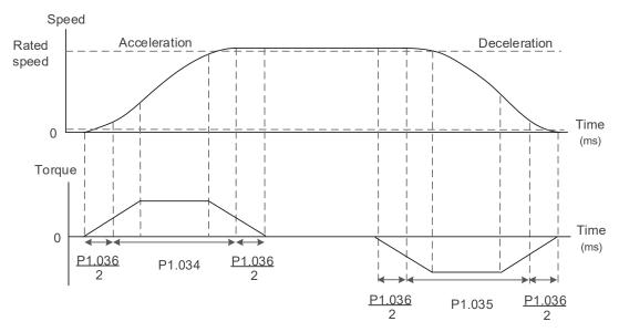
Figure 6.3.3.1 S-curve and time setting
