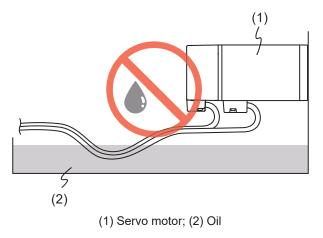
2. If oil or water is unavoidable, use oil-resistant cables. Delta does not provide oil-resistant cables.
