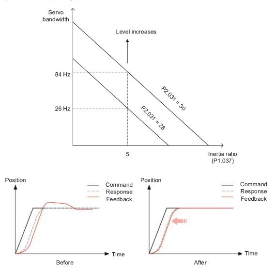
Figure 5.3.5.1 Adjust the bandwidth response level
