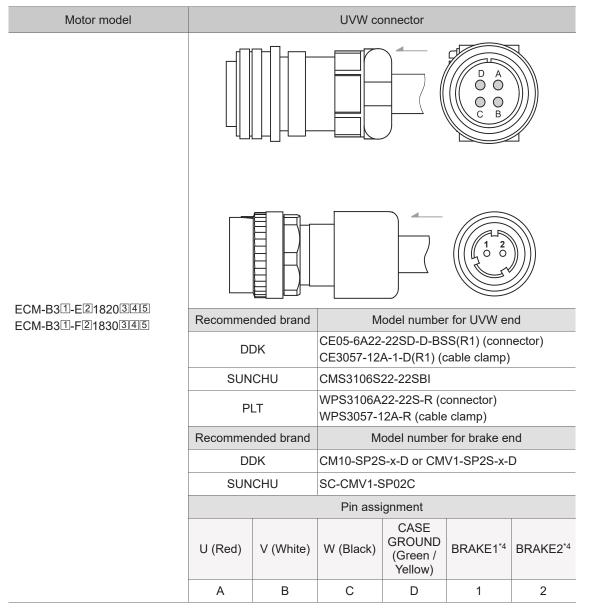
Wire selection: use a 600  $V_{\text{AC}}$  PVC cable. Refer to Section 3.1.6 for more information.
