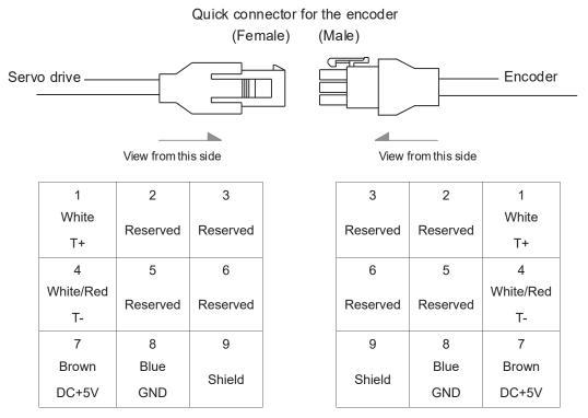
Note: the wire colors of the ASDA-B3 servo drive are for reference only. Refer to the actual servo drive.
