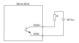
C6: DO wiring - the servo drive uses an external power supply and the resistor is for inductive load.
