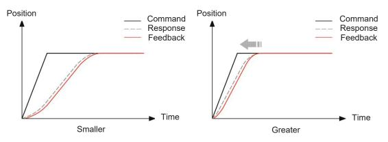
Figure 5.3.6.1 Adjust the command response gain
