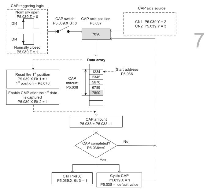
Figure 7.2.2.1 Flowchart for high-speed position capturing
