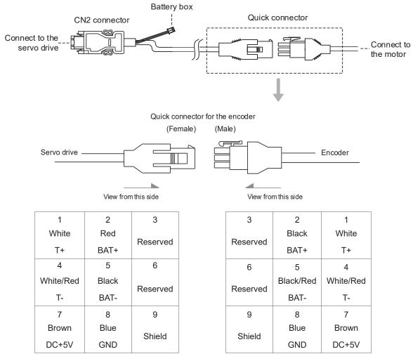
Note: the wire colors of the ASDA-B3 servo drive are for reference only. Refer to the actual servo drive.
