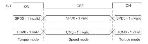
In Torque mode (DI.S-T is on), you select the Torque command with DI.TCM0 and DI.TCM1. When switching to Speed mode (DI.S-T is off), you select the Speed command with DI.SPD0 and DI.SPD1. The motor operates according to the Speed command. When DI.S-T is on, it returns to the Torque mode. Refer to the introduction of single mode for the DI signal and the selected commands for each mode.
