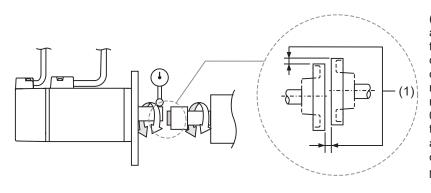
(1) The distance is measured at four different positions on the circumference for the centering precision. The difference between the maximum and minimum measurements should be 0.03 mm or less; even within this range, you can make adjustments to increase the centering precision.
