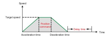
Figure 7.1.3.3.2 Parameters for PR mode position control
