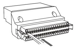
The CN1 quick connector has multiple spring terminals. Determine which terminal is to be wired in advance. Use a flathead screwdriver to press the spring down to open the pin.
