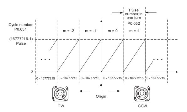
Figure 10.3.2.1 Absolute position for pulse number
