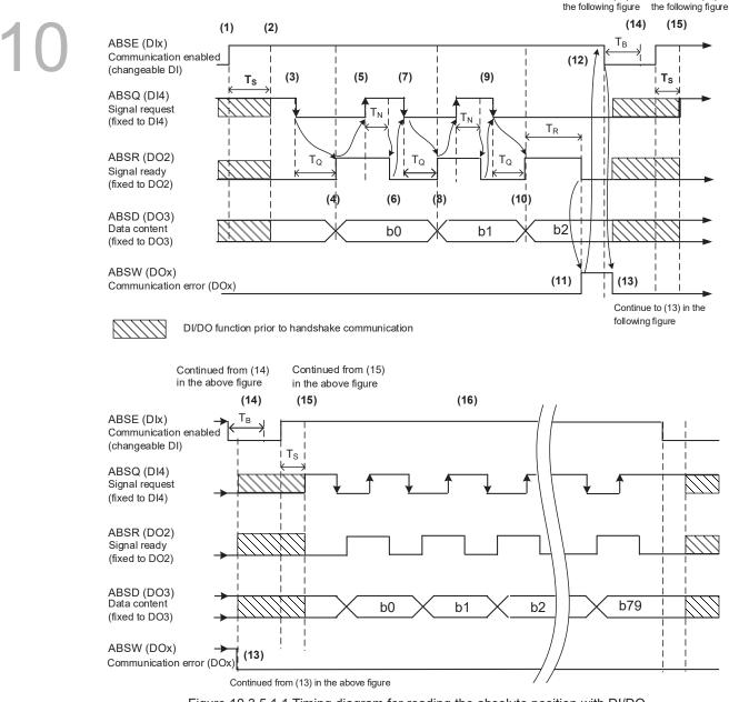
Figure 10.3.5.1.1 Timing diagram for reading the absolute position with DI/DO
