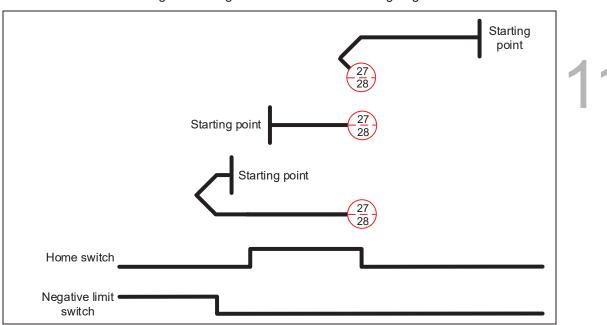
Methods 27 and 28: homing on the negative limit switch and falling edge of home switch
