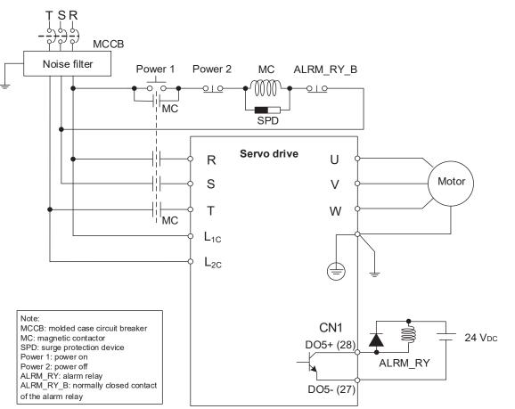
■ Wiring method for three-phase power supply (for all series)
