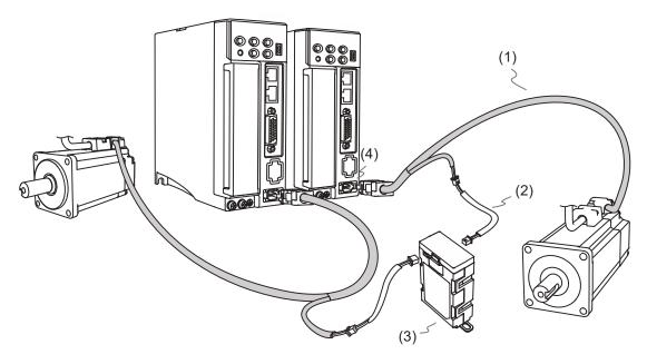
(1) Encoder cable; (2) Battery box cable AW; (3) Dual battery box (absolute type); (4) CN2 connector
