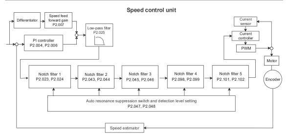
The ASDA-B3 provides two types of resonance suppression: one is the Notch filter and the other is the low-pass filter. See the following diagrams for the results of using these filters. System open-loop gain with resonance:
