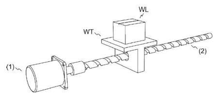
(1) Motor; (2) Ball screw pitch: 3 mm (equals 3,000 µm); WL: workpiece; WT: platform
