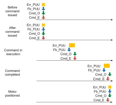
Figure 7.1.3.1.3 Homing mode and monitoring variables
