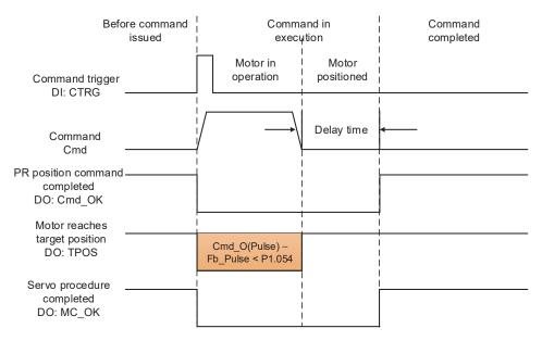
Figure 7.1.2.4 Operation of DI/DO signals in PR mode (including delay time)
