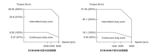
Note: in the servo motor model name, 2 represents the encoder type; 3 represents the brake or keyway / oil seal type; 4 represents the shaft diameter and connector type; and 5 represents the special code.
