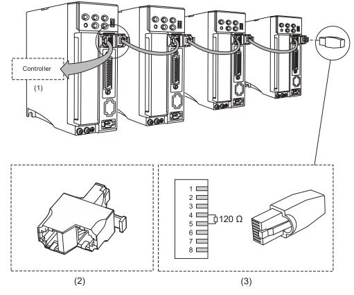
(1) Connect to the controller / PLC; (2) Modbus connector; (3) Wiring for RS-485 terminal resistor
