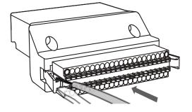
(2) Insert the stripped wire into the pin and withdraw the screwdriver to complete the wiring.
