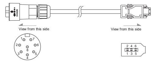
Pin assignment of CN2 connector:
