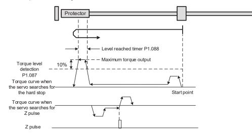
Note: the actual maximum torque output of the motor is 10% greater than the detected torque level (P1.087).
