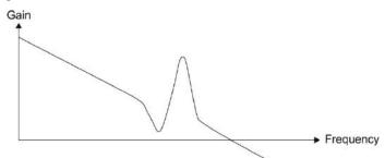
When the value of P2.025 is increased from 0, BW becomes smaller, as shown in the following figure. Although it solves the problem of the resonance frequency, the response bandwidth and phase margin are reduced.
