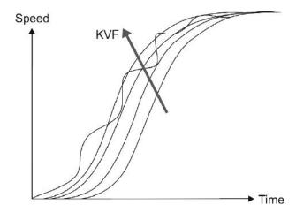
The closer the KVF value is to 1, the more complete the forward compensation. The following error becomes very small. However, a KVF value that is set too high also causes vibration.
