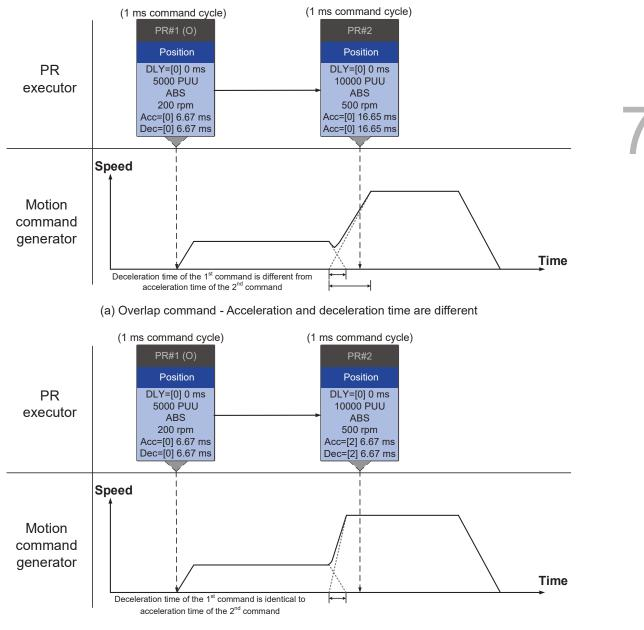
(b) Overlap command - Acceleration and deceleration time are identical
