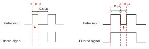
If the first pulse width is smaller than 0.8  $\mu$ s, it may be filtered out, and thus two input pulses will be regarded as one pulse. If the pulse width is smaller than 0.2  $\mu$ s, it will be filtered out. If the low level pulse width is smaller than 0.8  $\mu$ s, it may be filtered out, and thus two input pulses will be regarded as one pulse. If this low level pulse width is smaller than 0.2  $\mu$ s, it will be filtered out.
