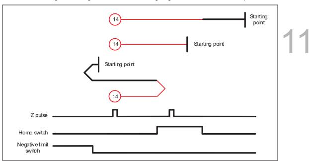
Method 14: homing on the negative limit switch, rising edge of home switch, and Z pulse
