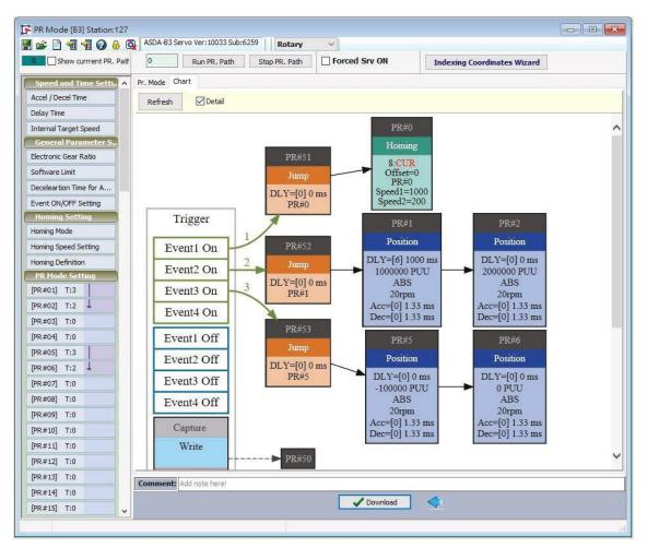
Figure 7.1.3 PR Diagram display in ASDA-Soft
