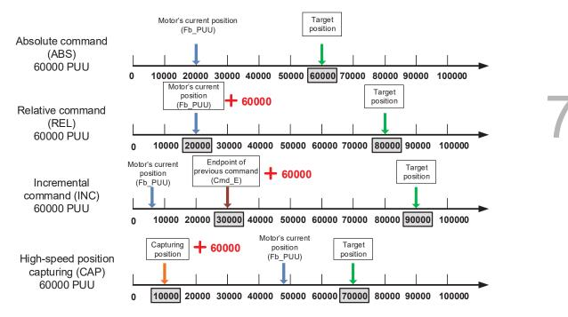
Figure 7.1.3.3.3 Four types of Position command
