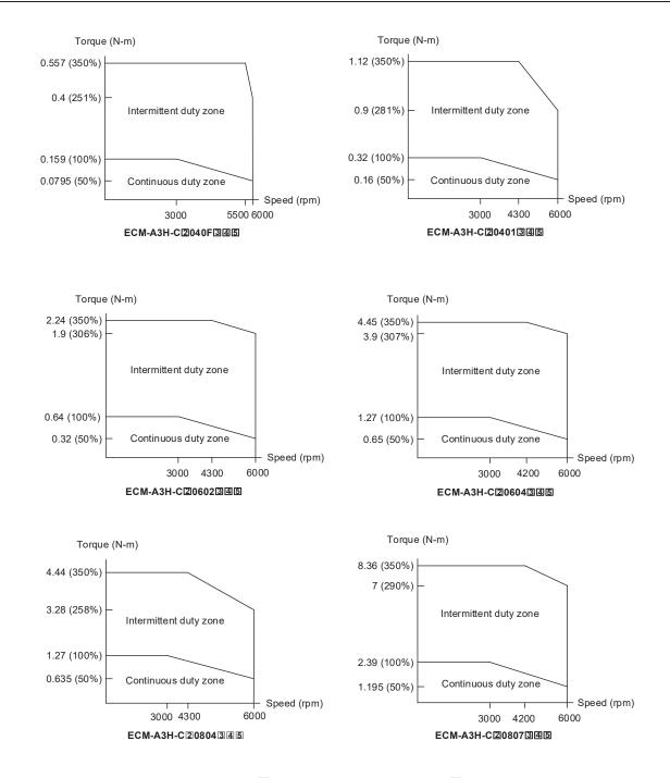
Note: in the servo motor model name, 2 represents the encoder type; 3 represents the brake or keyway / oil seal type; 4 represents the shaft diameter and connector type; and 5 represents the special code.
