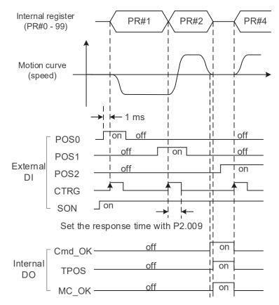
Note: Cmd\_OK is on when the PR command is complete; TPOS is on when the error is smaller than the value set by P1.054; MC\_OK is on when Cmd\_OK and TPOS are both on.
