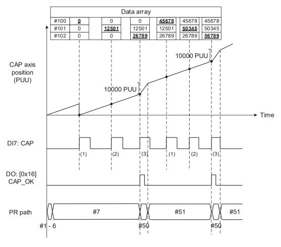
Figure 7.2.2.4 Application example for high-speed capture function
