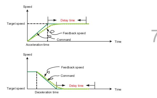
Figure 7.1.3.2.2 Parameters for PR mode speed control
