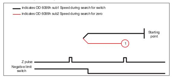
Method 2: homing on the positive limit switch and Z pulse
