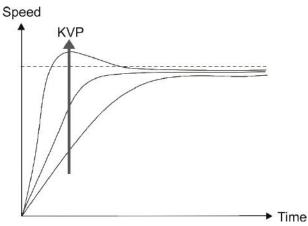
The higher the KVP value, the larger the bandwidth. The time of the speed increase will also be shorter. However, if the value is set too high, the phase margin is too small. The effect is not as good as KVI for the steady-state error but is better for the effect on following error.
