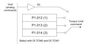
When using the Torque Limit function, set this parameter to 1 to limit the torque permanently without occupying a DI setting. Alternatively, you can enable or disable the limit function with DI.TRQLM, which is more flexible, but the setting then occupies a DI setting. You can enable the Torque Limit function with either P1.002 or DI.
