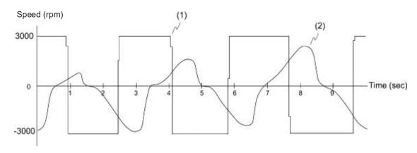
(1) Analog Speed command; (2) Motor speed
