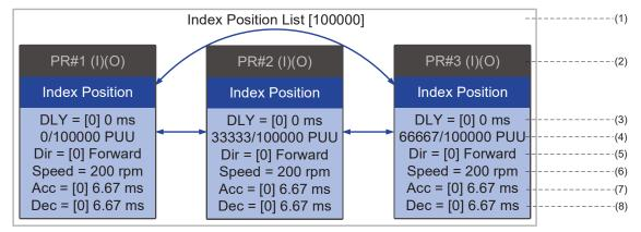
Figure 7.1.4.7 Index Position command display
