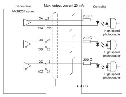
Note: the pin definition of the communication type models is different from that of the L model. Communication type model pins: OA (1), /OA (2), OB (11), /OB (12), OZ (3), and /OZ (4). C11: encoder OCZ output (open collector Z pulse output)
