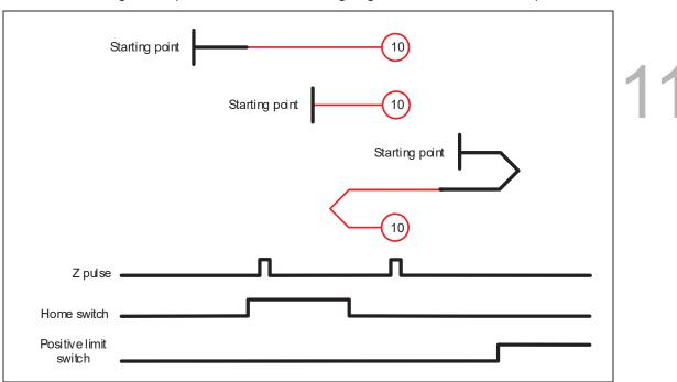
Method 10: homing on the positive limit switch, falling edge of home switch, and Z pulse
