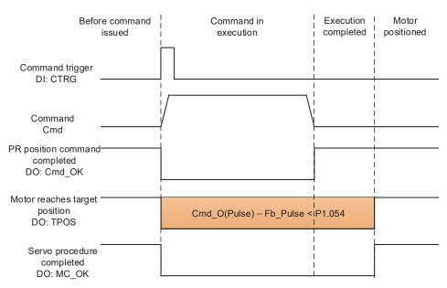
Figure 7.1.2.3 Operation of DI/DO signals in PR mode
