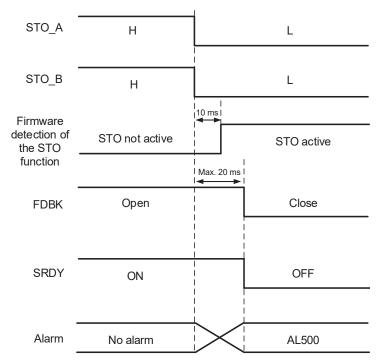
**AL501 / AL502:** see the following diagram. When the motor runs normally, but one of the safety signal source is low for 1 s, the firmware disables the drive (Servo Off) and triggers AL501 or AL502. The following diagram illustrates AL501.
