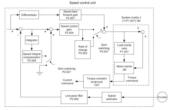
In the speed control unit, you can adjust different types of gain. You can adjust the gain manually or use the two gain adjustment modes provided.
