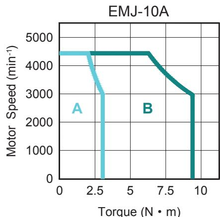
A: Continuous Working Area    B: Repeatable Working Area
