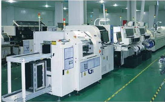
SMT Chip Mounter Machine Production Line
