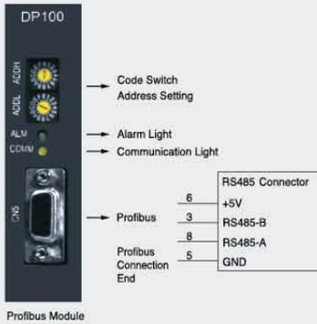
There are many applications based on profibus communication in industrial automation market. DP100 module is a PROFIBUS DP module, which can connect the other PROFIBUS products with ESTUN ProNet servo drive, and the project cost of providing profibus connection is low.
