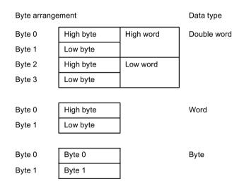
Figure 9-9 Byte arrangement in "big endian" format
