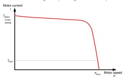
Figure 2-1 Typical starting current characteristic of a three-phase asynchronous motor
