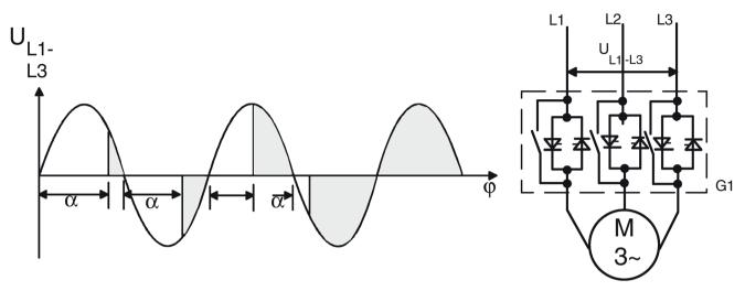
Figure 2-5 Phase angle control and schematic diagram of a soft starter with internal bypass contacts
