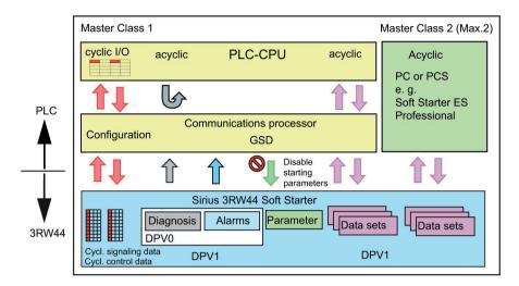
Figure 9-2 Communication principle
