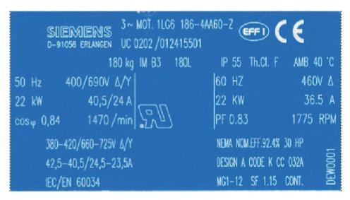
Figure 4-4 Nameplate of a 22 kW motor
