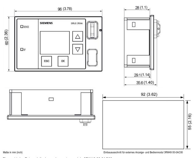
Figure 11-4 External display and operator module 3RW49 00-0AC00
