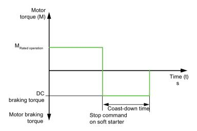
Figure 7-9 DC braking
