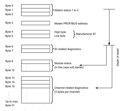
Figure 9-4 Structure of the slave diagnostics
