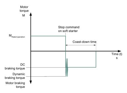
Figure 7-8 Combined braking
