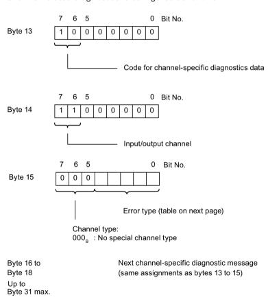
Figure 9-7 Configuration of the channel-related diagnostics
