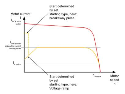
Figure 7-5 Current limiting with soft starter
