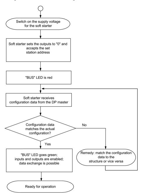
Figure 9-3 PROFIBUS DP starting of the soft starter
