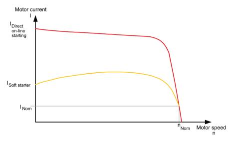
Figure 2-3 Reduced current characteristic of a three-phase asynchronous motor during startup with a SIRIUS 3RW44 soft starter
