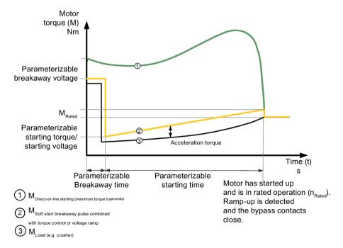
Figure 7-4 Function principle of torque control breakaway pulse
