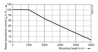
Figure 3-2 Reduction as a function of the installation altitude
