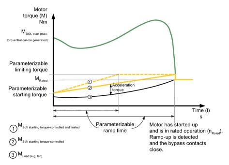
Figure 7-3 Function principle of torque control
