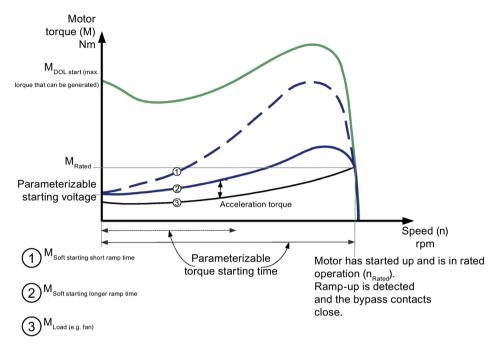
Figure 7-2 Principle of the voltage ramp for the torque characteristic
