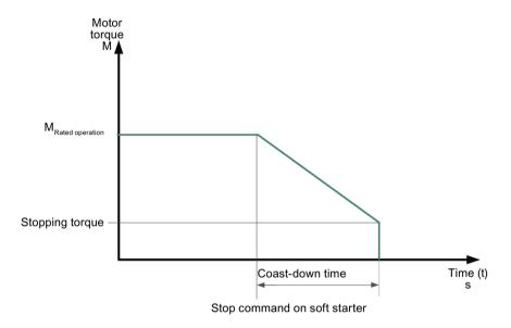
Figure 7-7 Soft stop/pump stop
