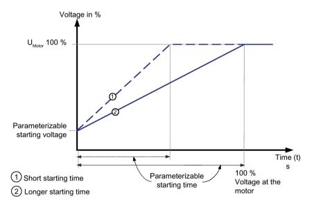
Figure 7-1 Function principle of the voltage ramp
