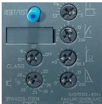
Easy setting via invariably adjustable rotary potentiometers
